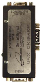
RS 232 Interface Adapter The adapter provides connections to a PC, the encoder system and the controller.
